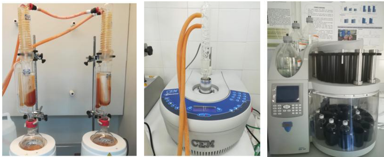
Figure 2. Comparisons of classical extraction methodologies (soxhlet) with new alternatives: microwave assisted extraction (MAE) or accelerated solvent extraction (ASE) system (from left to right). Source ICSURO
